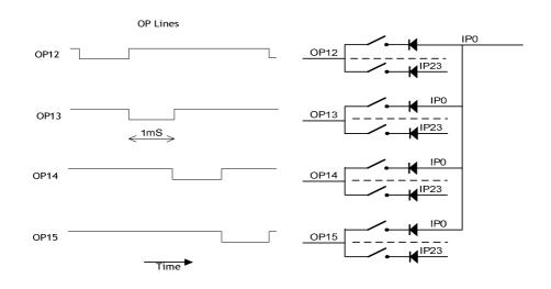
The function GetMultiplexedInputs returns the state of the multiplexed inputs. The data is returned as the following structure (which is defined in 'x10io.h'):
