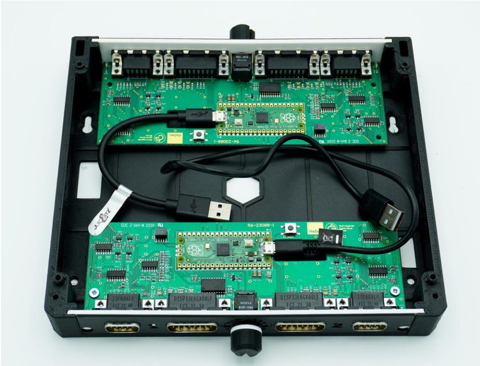
Two CTRLDock modules can be fitted, or the remaining internal space and removable back panel can be used for an optional SDD/HDD or other storage device or additional controller connection.
