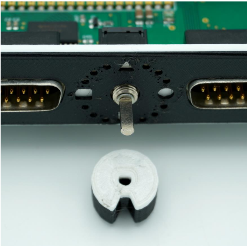
Fit the panel and rotate the switch so the flat face is directly up (this is Position Zero).
