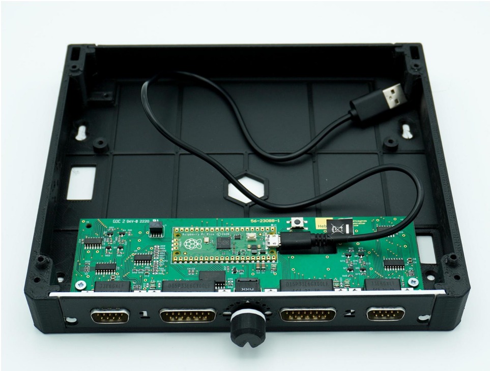
The CTRLDock Classic can be fitted into a Slice tray for the Multisystem
