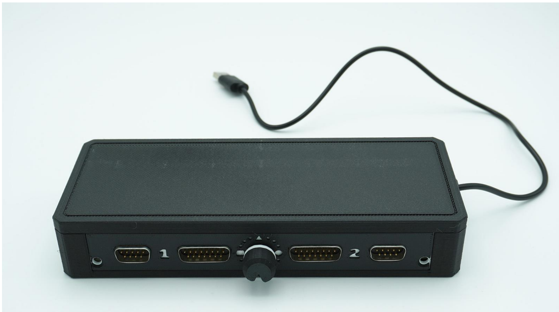
DE9/15 PCB in optional 3D printed enclosure (stand-alone USB)
